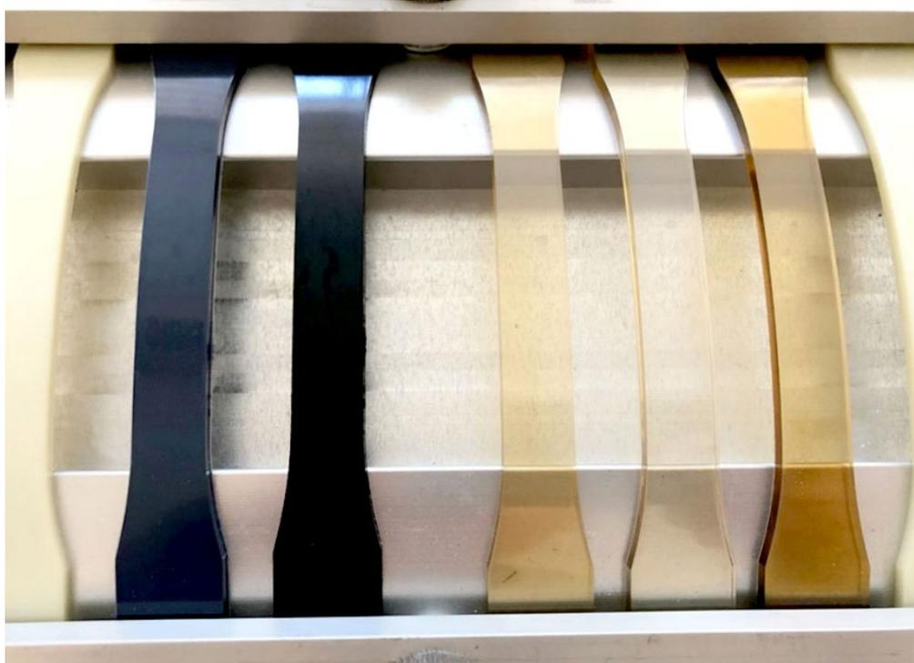
Figure 1. Tensile bars under flexural strain.
