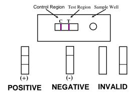
**Positive**: If both the C line and T line appear in the viewing area, the test indicates that HCG is present in the specimen at the level close to or higher than 25 mIU/ml.
